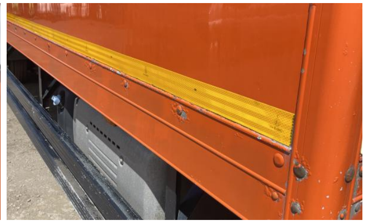
4: Door Moulding osf Scuffed (Unpainted) Over 100mm
