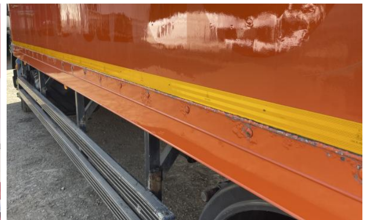
6: Qtr Panel osr Rusted Over 5mm
