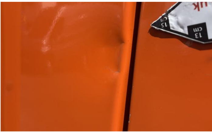
3: Door osf Dented With Paint Damage
