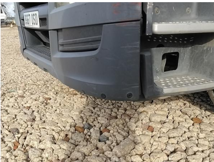
7: Bumper Front Moulding Scuffed (Unpainted) UpTo 100mm
