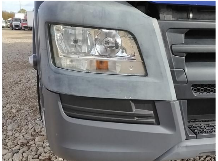
4: Fog Lamp Surround os Scuffed (Unpainted) UpTo 100mm
