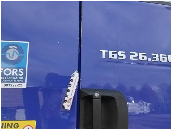
16: Door osf Chipped Edge Chip
