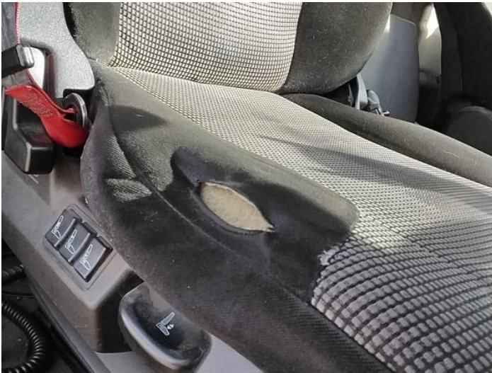
17: Seat Base Cover osf Holed Over 3mm
