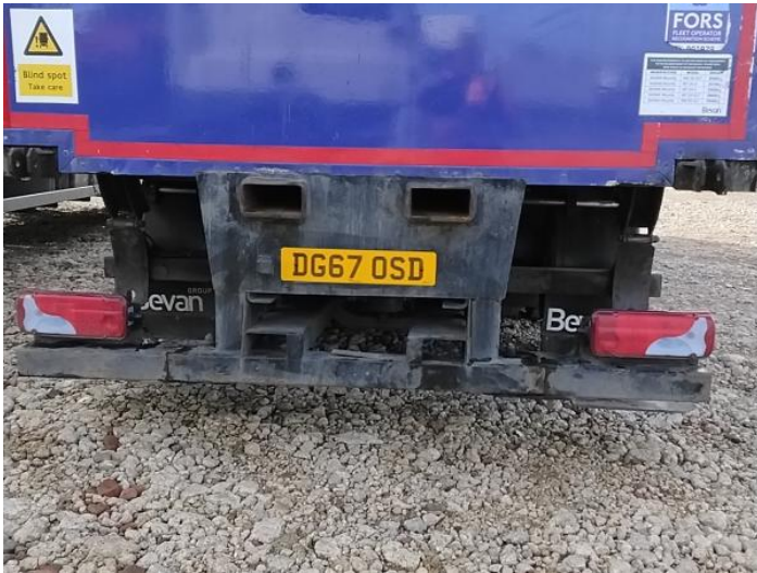
12: Bumper Rear Rusted Over 5mm
