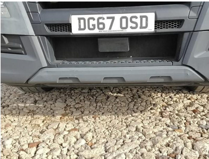
5: Bumper Front Moulding Scuffed (Unpainted) UpTo 100mm
