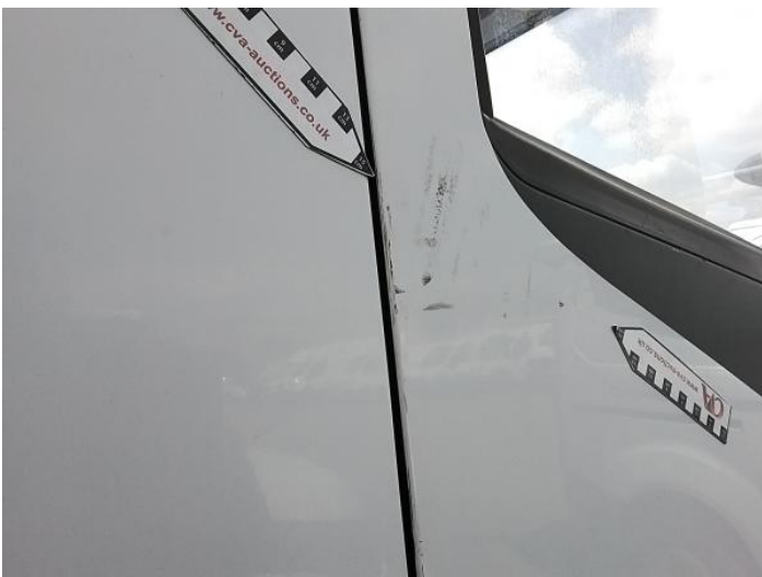
7: Door osf Scratched Over 25mm Thru Paint
