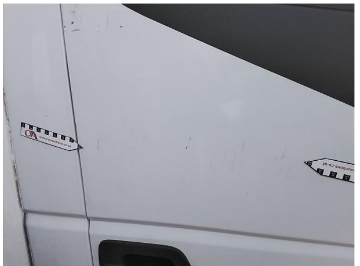
8: Door osf Scratched Over 25mm Thru Paint
