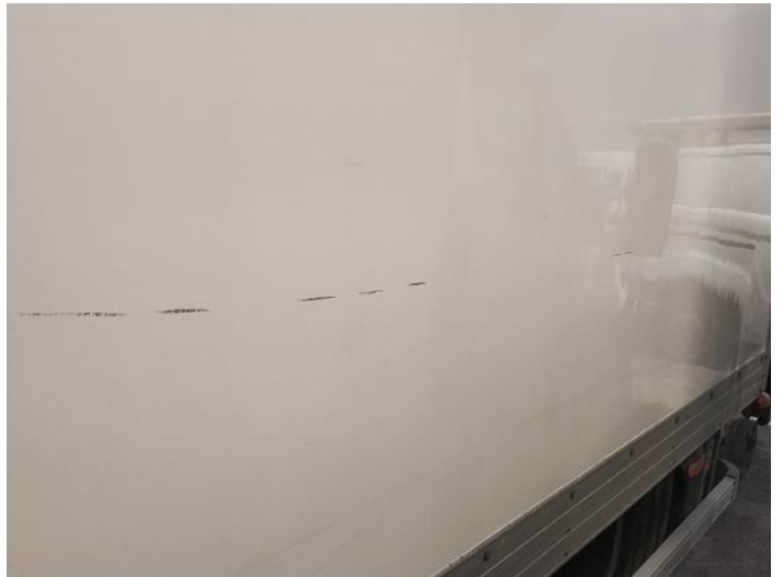
6: Qtr Panel osr Scratched Over 25mm Thru Paint
