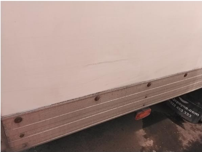
5: Qtr Panel osr Scratched Over 25mm Not Thru Paint
