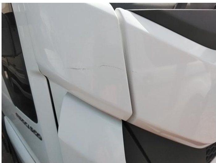
1: Panel Front Scratched Over 25mm Not Thru Paint
